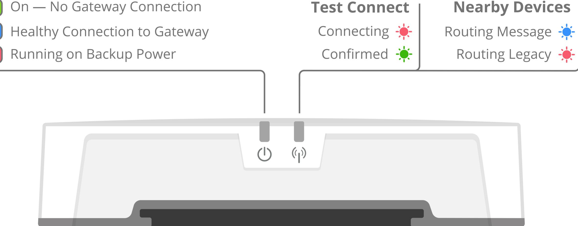
Note: After the Test Connect button is pressed, two slow blinks of the RF Activity LED show whether the Gateway can be reached. Fast blinks will occur at any time as signals are received from nearby NextCentury devices.
